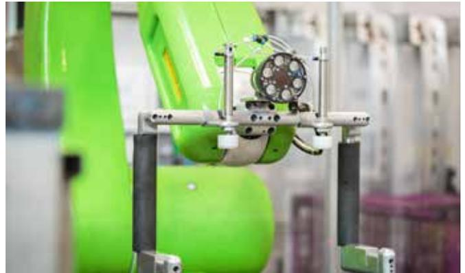
in the market. There are several components that weigh more than seven or ten kilograms, “laboratory robots” could not compete. The FANUC robot, which is based on the M-20iA series, has a reasonable reach of 1.813 mm regarding industrial applications.
